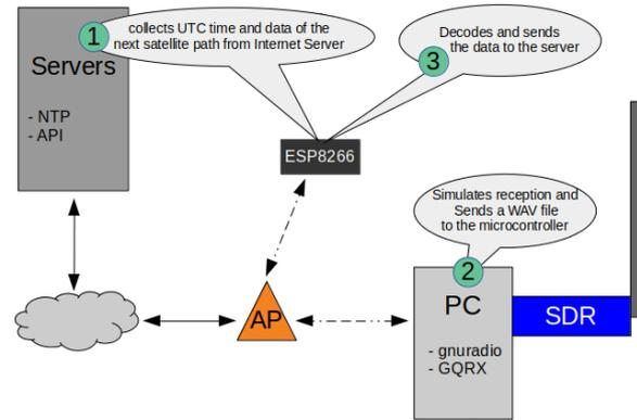
Figure 1: Global Architecture with the Wi-Fi microcontroller ESP8266.
