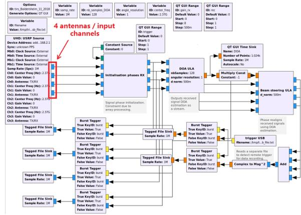
Figure 1: Flowgraph runnable at 1MS/s but creating data overflows at 8.33MS/s.
