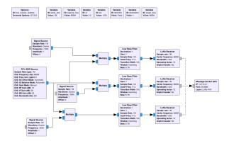
Figure 1: GNU Radio flowgraph for capturing Lo-RaWAN communications on 3 channels
