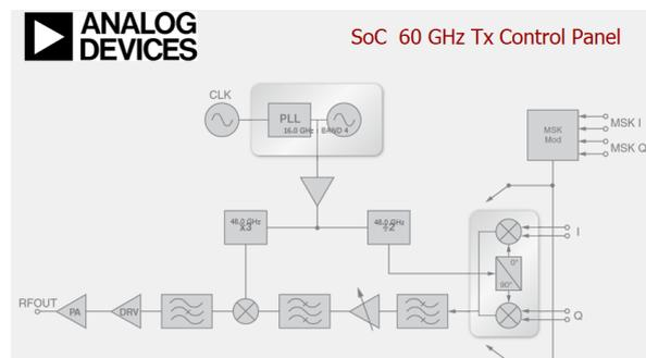
Figure 1: Block diagram of the HMC6300 SoC.
