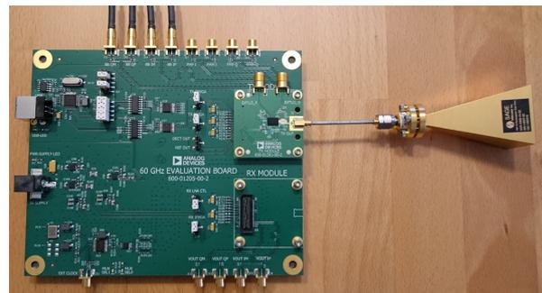
Figure 2: HMC6300 TX front-end fitted with SAGE horn antenna.
