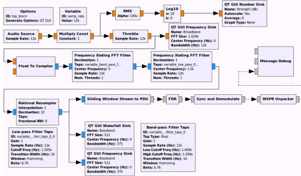
Figure 3: Flow graph of the audio decoder.
