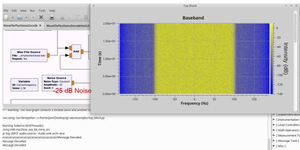
Figure 5: Decoding two frames with noise.
