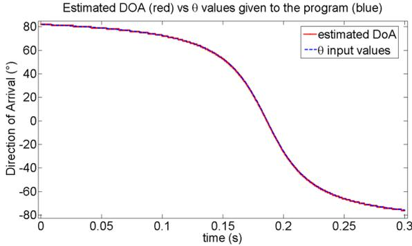
Figure 3: Estimated DOA (red) vs theta values fed to the program (blue) for the simulated trajectory.
