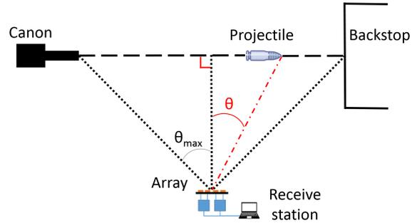
Figure 1: Proposed setup to electronically track a fired transmitting projectile with a passive ground-station steered by USRP
