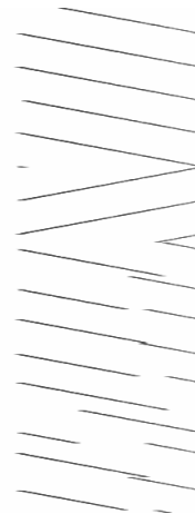
Figure 1. Spectrogram excerpt of a LoRa chirp y-axis: Time, x-axis: Frequency
