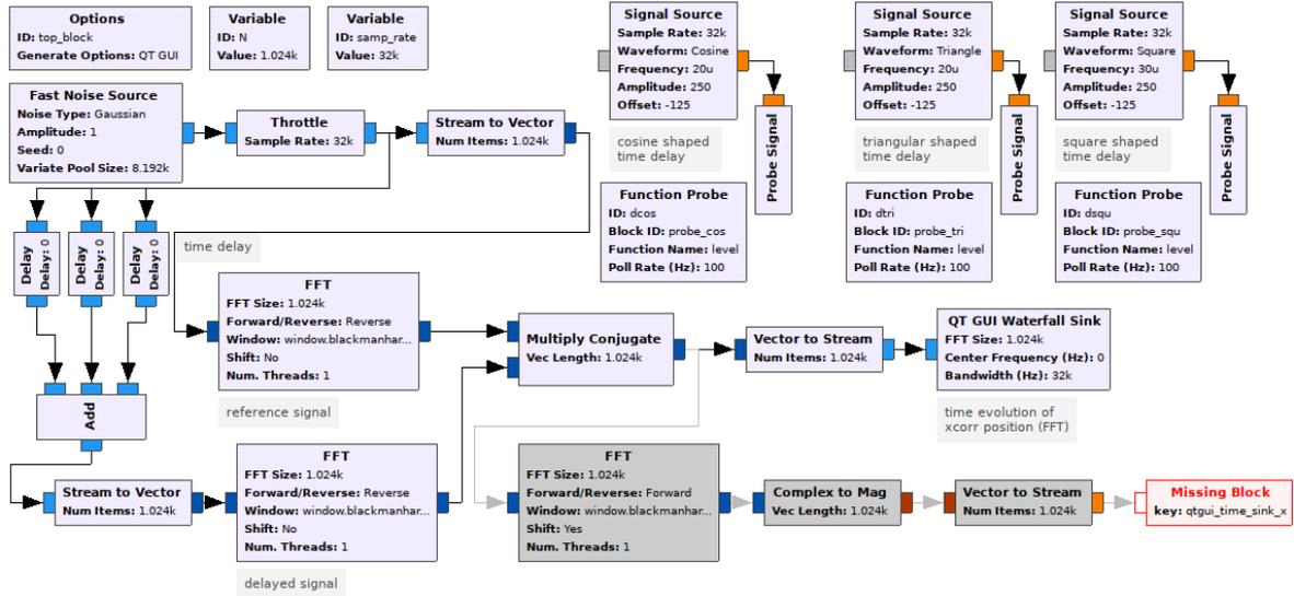
Figure 1: Real time computation of the correlation through the Fourier transform implemented in GNURadio: three delayed reference signal copies are generated using three different signal generators.
