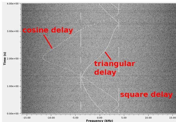
Figure 2: GNURadio Companion output with three targets delayed by square, sine and square wave time-delay functions visible on the waterfall. The data-rate constrained by the Throttle block is not constant, hence the shape deformation of the curves due to the varying speed.
