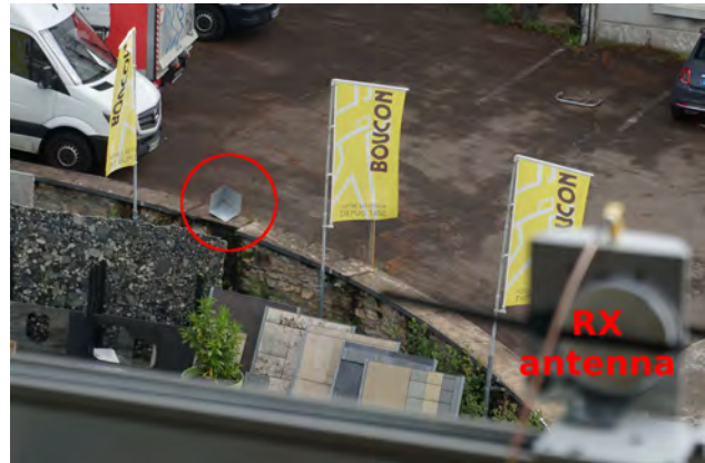
Figure 9. Corner reflector located at a range of 40 m of the RADAR setup, in front of car defining the needed RADAR cross section and hence cube side length of 30 cm.
