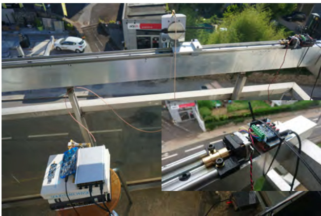
Figure 8. Motorized rail for reproducibly positioning with sub-mm accuracy the receiving antenna while keeping the emitting antenna static. Inset bottom-right: closeup on the lead-screw setup using a stepper motor controlled by a dedicated microcontroller receiving control commands through its USB (virtual serial) port.
