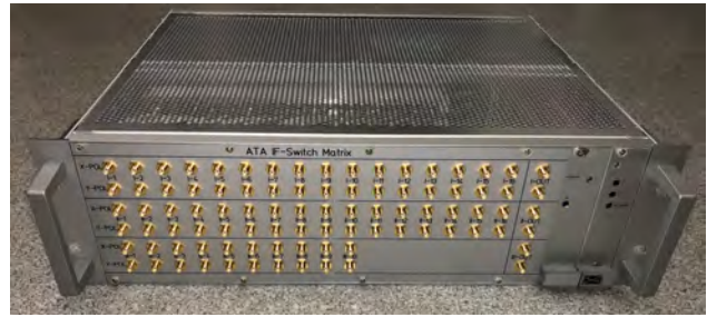
Figure 3. The ATA IF-Switch
