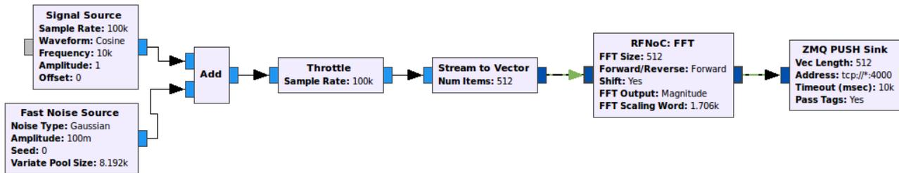
Figure 7. GNU Radio graph for the FFT block, target side.
