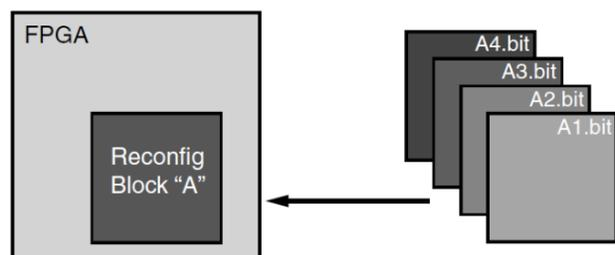
Figure 2. Partial Reconfiguration procedure, from (Xilinx, 2017c).
