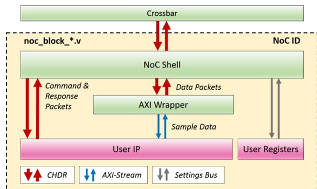
Figure 1. Internal structure of an RFNoC block, from (M. Braun, N. Cuervo, 2016).
