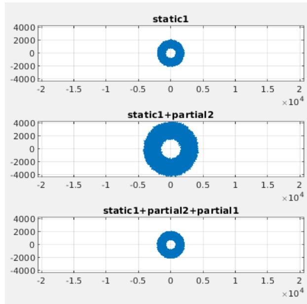
Figure 4. Testing the Partial Reconfiguration design with RFNoC Gain blocks in run-time. Gain1 block in the upper figure, Gain2 in the middle figure, Gain1 in the lower figure.
