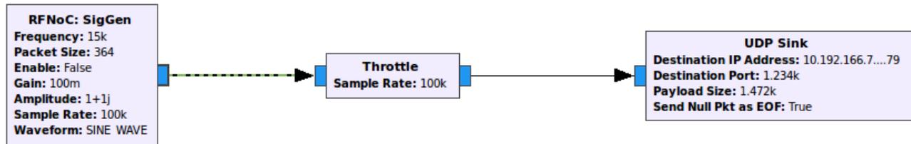
Figure 8. GNU Radio graph for the SigGen block, target side.
