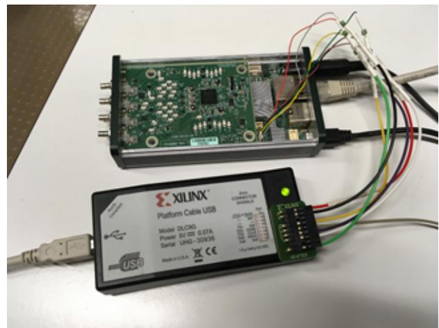
Figure 3. Writing the bitstreams to the FPGA of the E310 using a JTAG connector.
