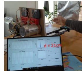
(b) Detected a target slowly moving in, with histogram position changed (indicating a moving “human/object” behind the wall)
