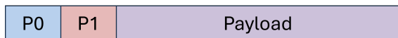
Figure 3. Packets are transmitted simultaneously by both radios such that only the payloads overlap. Each radio prepends its payload with its unique identifying pilot symbol in its assigned pilot slot (P0 or P1), thereby providing a brief “quiet” period that would allow for high-fidelity SI measurement.
