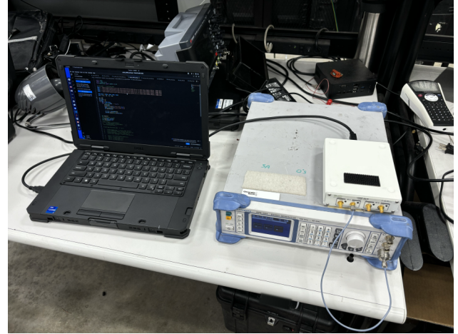
Figure 5. Power calibration and test setup. The laptop performs the automated calibration by commanding the signal generator (R&S SM100A) to output signals at the specified frequencies and power levels. UHD power calibration utilities generate the calibration table.
