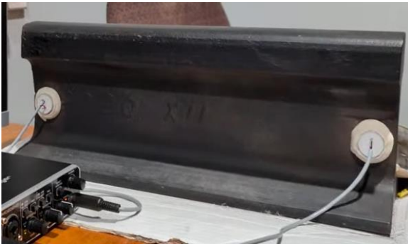
Figure 12 Steel Rail 60KG used in Sydney Trains network
