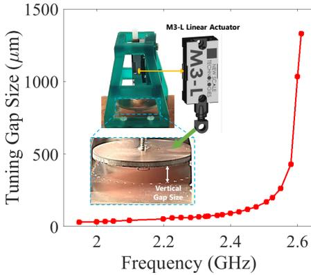
Figure 3. Measured tuning curve for the reconfigurable antenna. The center frequency of the antenna is tuned by vertically displacing the conductive disk across a large range of gap sizes.
