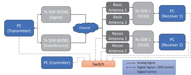
Figure 6. Extended Testbed Architecture (future)
