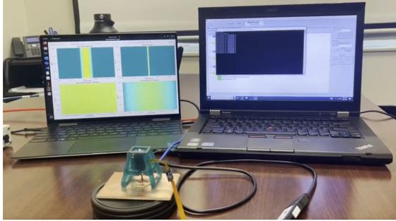
Figure 9. Physical deployment demonstrating control node (Windows PC, right) with New Scale Pathway software, the tunable antenna, and receive node (Linux PC, left) running GNURadio.
