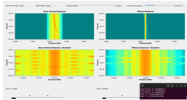
Figure 8. Simulation results showing automated configuration of signal and interference parameters via XMLRPC and power measurements via ZMQ (configured from Python script on the GNU-Radio computer via localhost connections).
