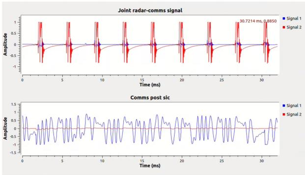
Figure 8. (upper) Joint radar-comms signal at the joint receiver end, (lower) result of the post SIC. Only communications signal with noise.
