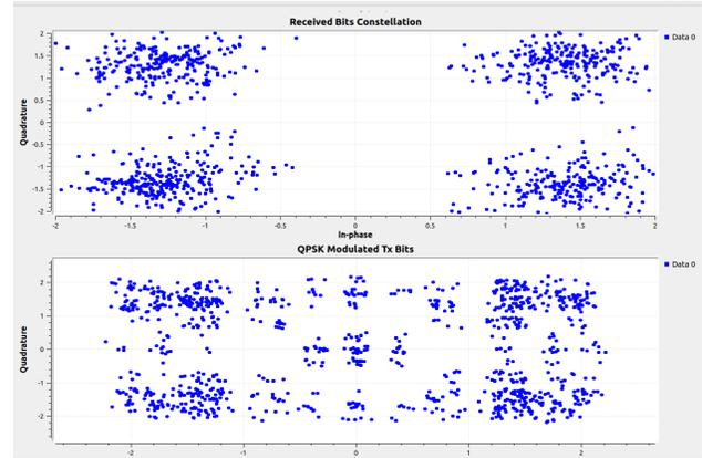
Figure 10. The constellation of the BPSK modulated header and the QPSK modulated message bits at the transmitting and receiving ends.
