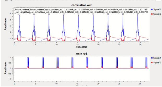
Figure 7. (upper) Output of the correlation estimator block and peak detection, (lower) only radar transmission.
