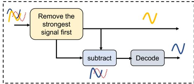
Figure 2. Simple block diagram of Successive Interference Cancellation algorithm SIC.
