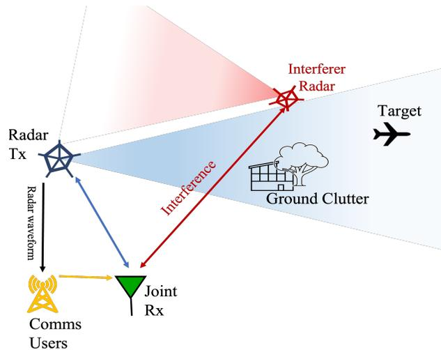
Figure 1. Example joint radar-communications system configuration in which a joint transceiver simultaneously receives transmissions from a radar transceiver, communications transceiver, and an interferer.
