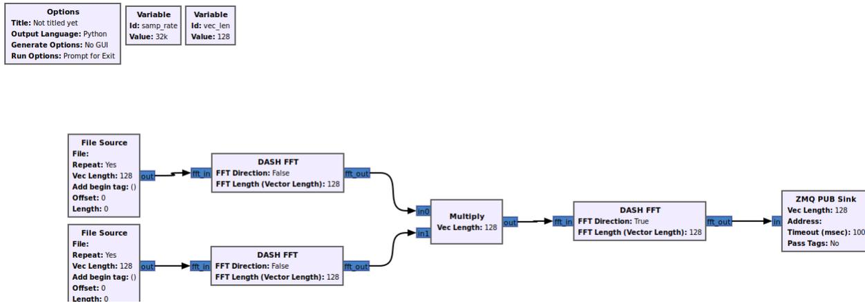
Figure 7. GNURadio Flow graph used for the radar correlator example application with run-time accelerator selection
