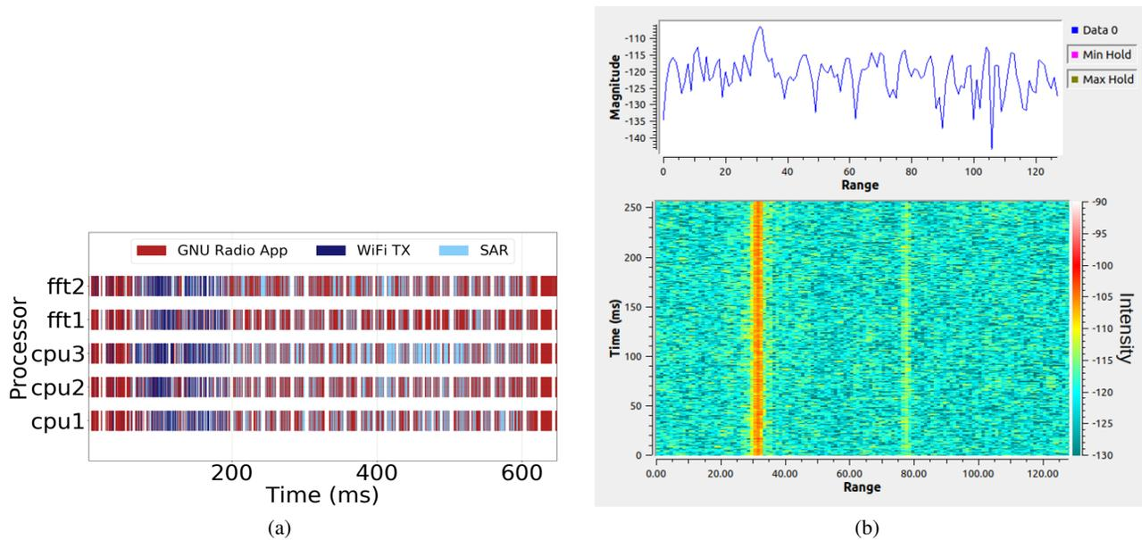
Figure 8. (a) GNU radio application (Radar Correlator) executing with dynamically arriving WiFiTx and SAR applications through CEDR on a SoC with 3 ARM cores and 2 FFT accelerators emulated on ZCU120 FPGA platform. (b) Waterfall image collected at runtime from CEDR based execution is identical to the output of the baseline implementation.
