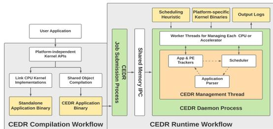
Figure 1. High level architectural overview of CEDR ecosystem.
