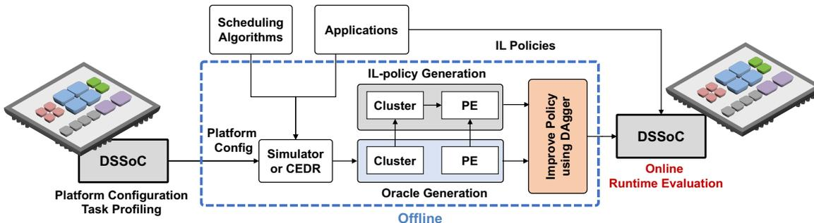
Figure 6. An overview of the IL-based Scheduling Framework.
