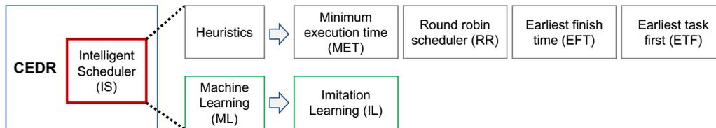
Figure 5. The intelligent scheduler (IS) framework integrates into CEDR and comprises a variety of heuristic and machine learning scheduling algorithms.
