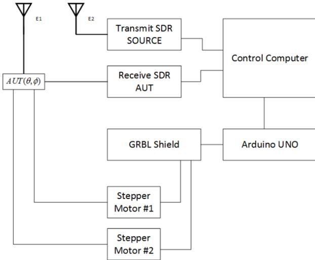
Figure 2. Block diagram of Antenna Pattern Measurement system.
