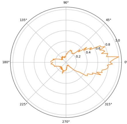
Figure 4. Example of 2.4 GHz Yagi prototype measured pattern using noise reduction method.
