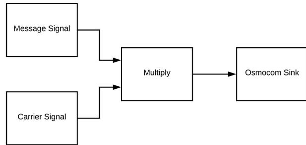
Figure 5. DSB-SC AM Transmitter Flow Chart.
