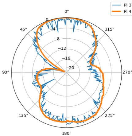
Figure 10. Raspberry Pi 3 vs 4 Patch Antenna.
