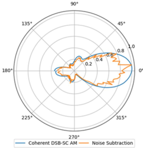
Figure 7. Measured principal plane pattern boresight ( $\Theta = 90^\circ, 180^\circ < \Phi < 180^\circ$ ) of the Yagi antenna prototype. Both the Coherent DSB-SC AM and Noise Subtraction methods are shown for comparison.
