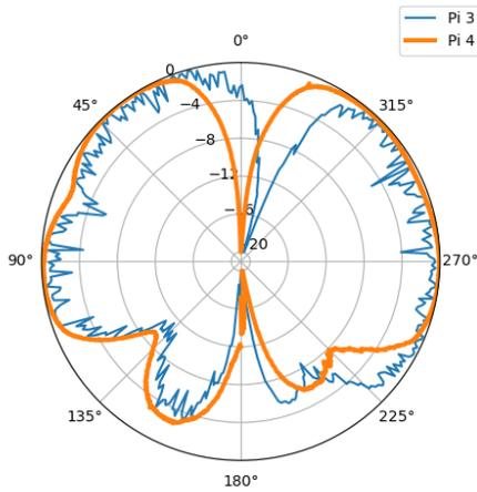
Figure 9. Raspberry Pi 3 vs 4 Mono-pole Antenna.
