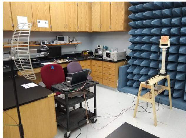
Figure 1. Antenna Pattern measurement system. Emphasis was placed on use of commercial PVC material with 3-D printer hardware including synchronous belts and gears
