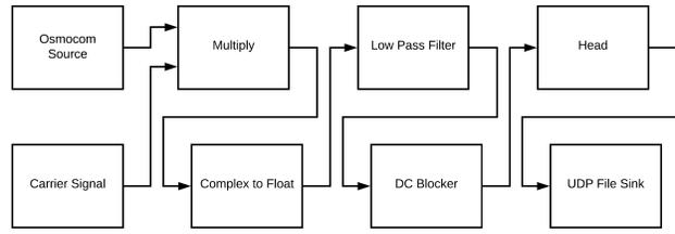
Figure 6. DSB-SC AM Receiver Flow Chart.
