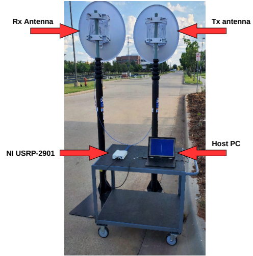
Figure 8. Experimental test bed setup
