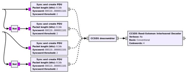
Figure 6. Tianwen-1 high speed decoder flowgraph (third section)
