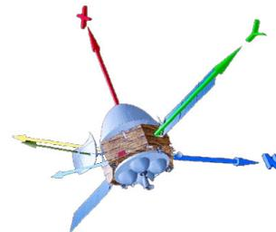
Figure 8. Tianwen-1 spacecraft body axes
