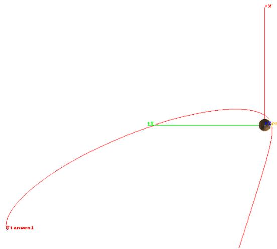
Figure 9. Tianwen-1 Mars orbit insertion simulated in GMAT
