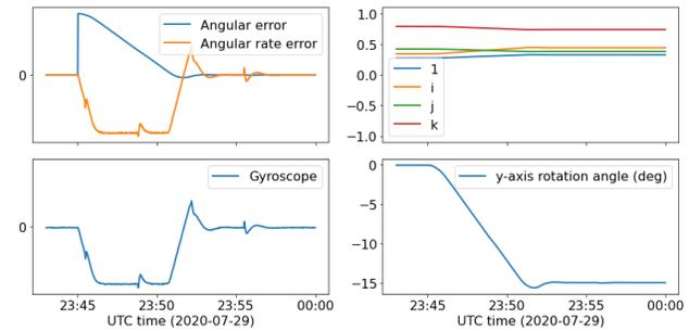
Figure 7. ADCS telemetry during  $-15^\circ$  rotation about  $y$ -axis
