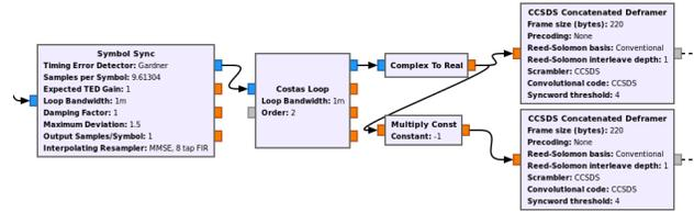
Figure 3. Tianwen-1 low rate decoder flowgraph (second section)
