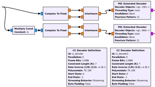
Figure 5. Tianwen-1 high speed decoder flowgraph (second section)
