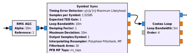
Figure 4. Tianwen-1 high rate decoder flowgraph (first section)
