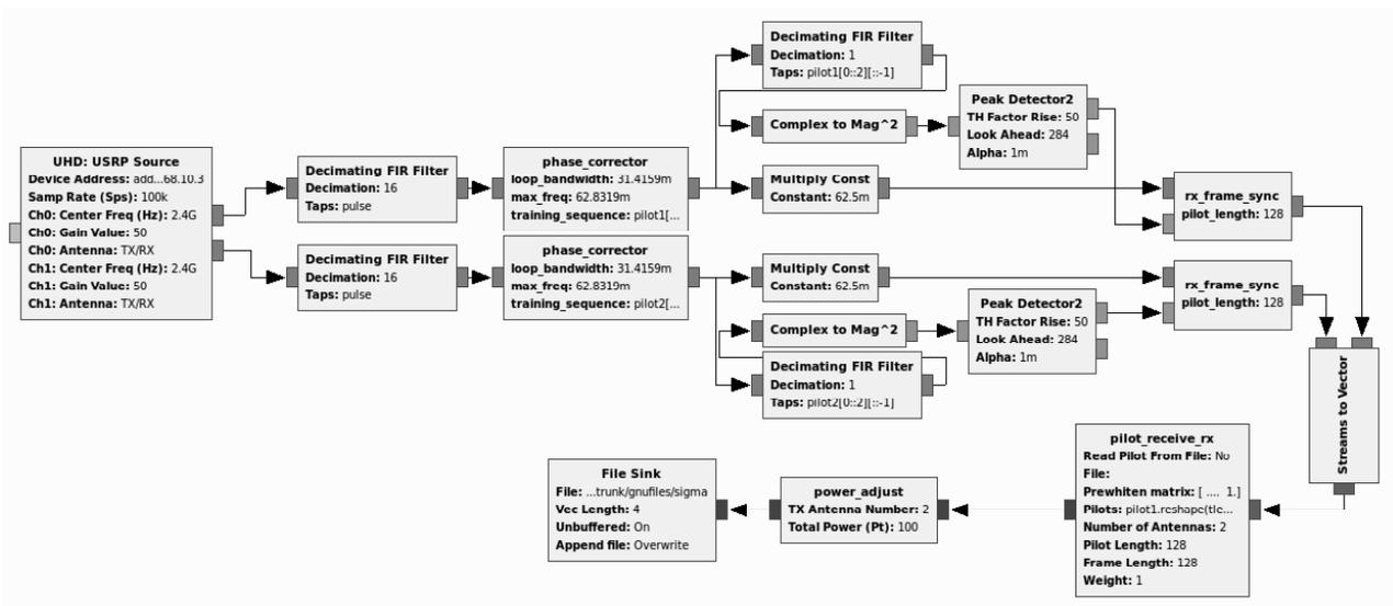
Figure 4. Rx of the E310 network mode
