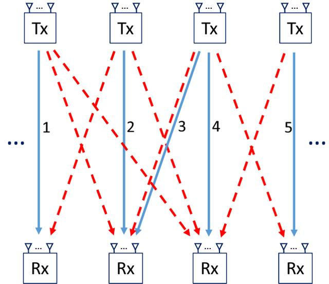
Figure 1. An example of B-MAC network. The solid lines represent data links and the dash lines represent interference.
