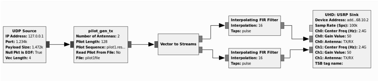
Figure 3. Tx of the E310 network mode
